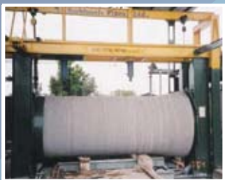
PSC Pipe Hydrostatic testing
