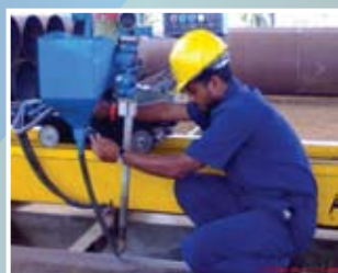
Sub Merged Arc Welding
